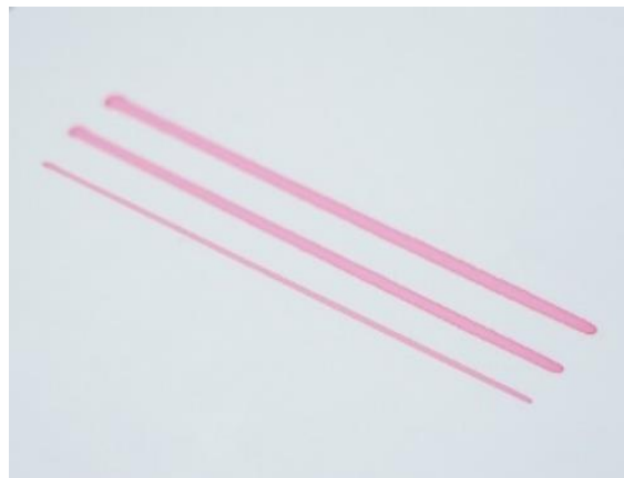
FIGURE 2: THE HOMOGENEOUS REAGENT LINES WERE PRINTED WITH DISPENSING PIPE ID 125-S-C (CHANNEL 1), ID 200-S (CHANNEL 2) AND ID 500-S (CHANNEL 3). THE REAGENT LINES CONSISTED OF 5, 10 AND 25 NANOLITER DROPLETS, RESULTING IN 0.5, 1 AND 2 MM LINE WIDTH, RESPECTIVELY.
